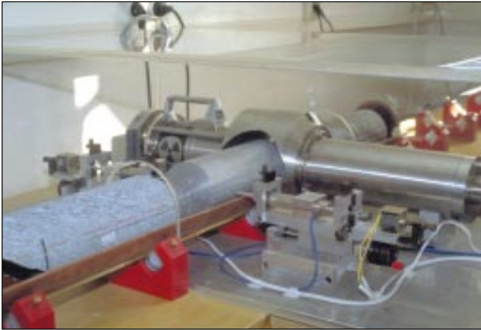
□ Field laboratory core measurements—detailed density profile (left) and electrical conductivity measurements (right).
